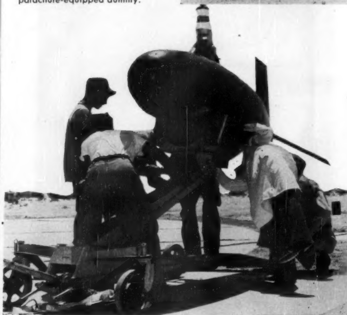
This weird looking merry-go-round rising over the California desert isn't a displaced piece of equipment from a touring carnival. Powered by a 2800-hp G-E motor, this tower can produce speeds up to 500 miles an hour, and is used to study the effect of centrifugal force on parachutes of pilots who bail out of crippled jet aircraft. Picture below shows airmen adjusting the gondola housing a parachute-equipped dummy.
